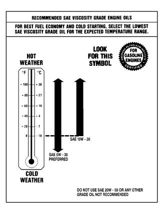
As in the chart shown previously, SAE 5W-30 is best for your vehicle. However, you can use SAE 10W-30 if it's going to be  $0^{\circ}$ F (-18°C) or above. These numbers on an oil container show its viscosity, or thickness. Do not use other viscosity oils, such as SAE 20W-50.
